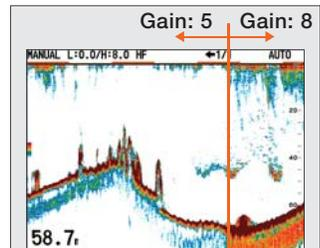
With conventional gain controls, changes are made for new echoes only when the gain setting is changed.
